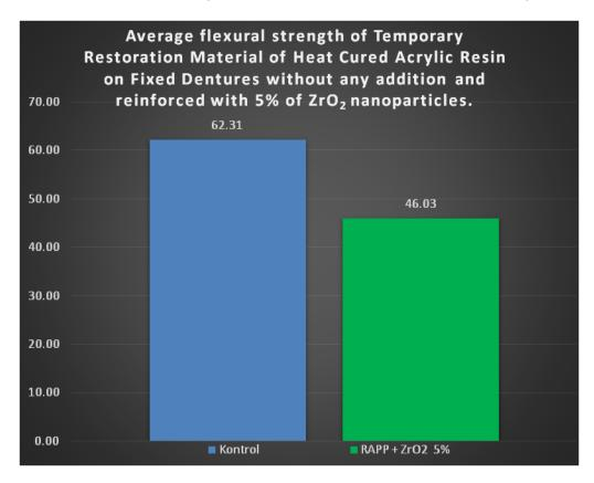
The effect of flexural strength on each test group is done with t-test. Normality and homogeneity tests are first done on this study and homogenity showed a value of p=0,65 (p>0,05) which means the data obtained is homogenous. Normality test value on this study is p>0,05 which means all the data are normal.
