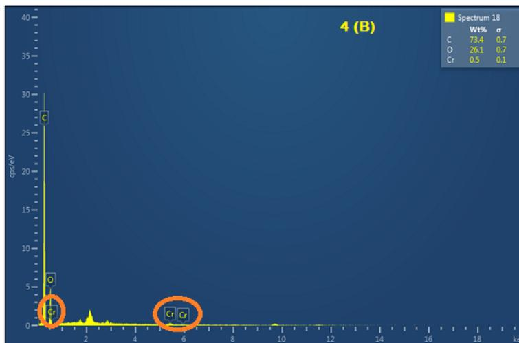
Fig. 4: EDAX images (A) before and (B) after adsorption of total chromium by APP
