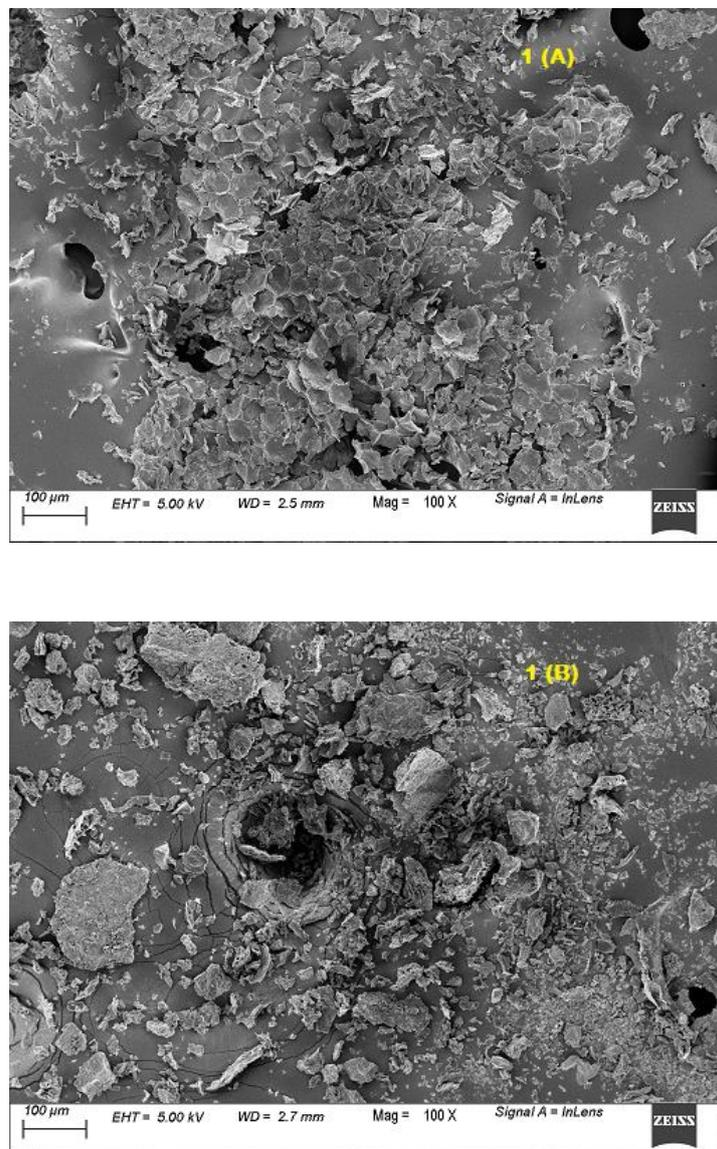
Fig. 1: SEM images (A) before and (B) after adsorption of total chromium by AGP
