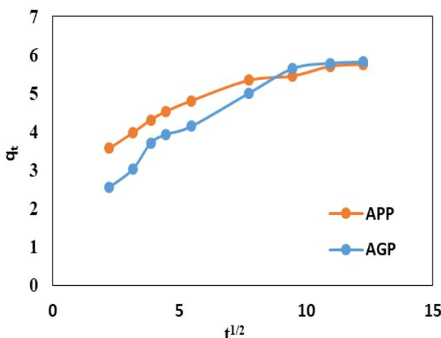
**Fig. 5: Intra – particle diffusion model plot for chromium adsorption by AGP**
