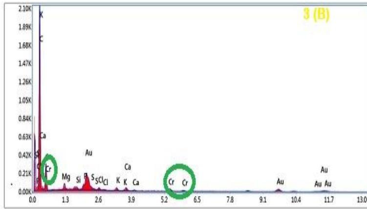
Fig. 3: EDAX images (A) before and (B) after adsorption of AGP
