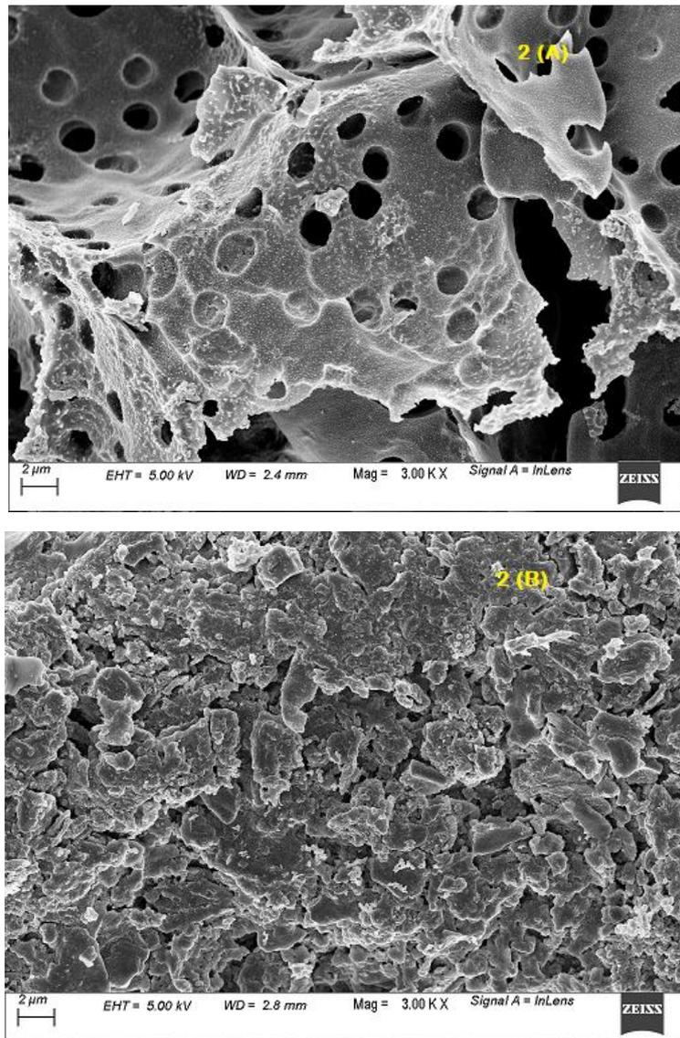
Fig. 2: SEM images (A) before and (B) after adsorption of total chromium by APP
