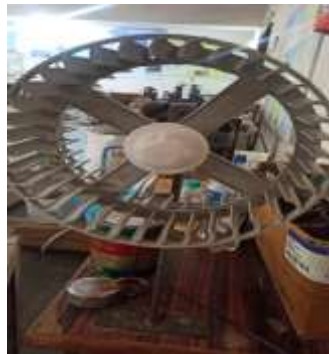
Fig.4: covering the blower front portion with a cap so that the blower will not move axially
