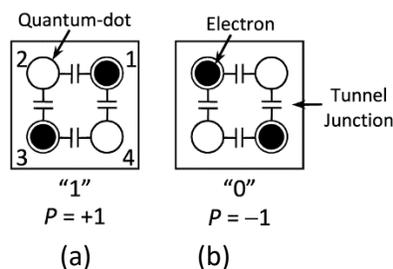
By connecting the cells in cascade, a QCA wire is formed [9]. The polarization that is logic 1 or logic 0 is formed by tunnelling of two electrons. This information is in the form of columbic charge only as depicted in Figure 2.
