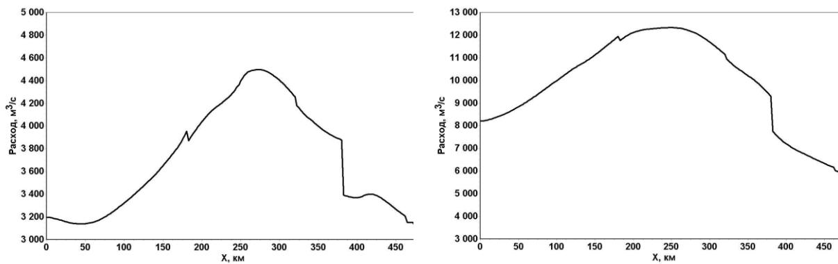
Figure: 1. Calculated distribution of discharge along the river bed. Tupalang at the time of the maximum water level near Sariasia according to 2017 (a) and 1997 data. (b). X coordinate values correspond to: 0 - Sariasia; 239 - Denau; 481 - village Shurchinskoe
