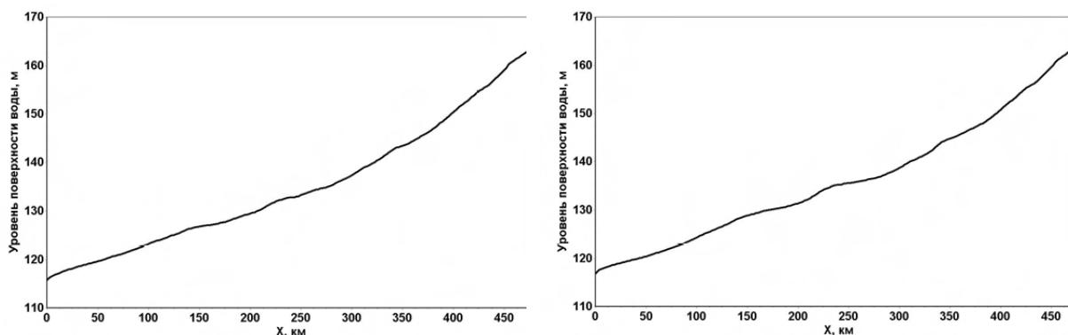
Fig. 2. The calculated distribution of the water surface level along the river. Tupalang at the time of the maximum water level near the city of Sariasia according to data from 2017 (a) and 1997. (b). X coordinate values correspond to: 0 - Sariasia; 239 - Denau; 481 - village Shurchinskoe.
