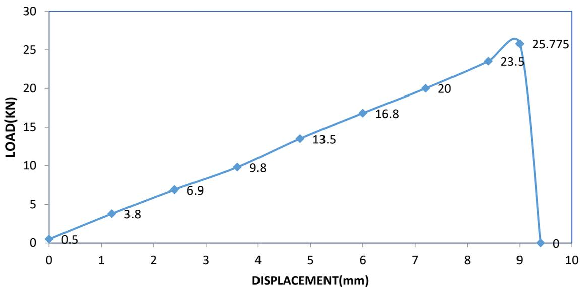
Figure 4 Tensile Properties of Stitched Plates
