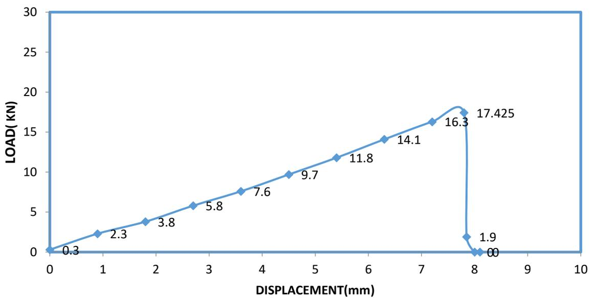
Figure 3. Tensile Properties of Unstitched Plates
