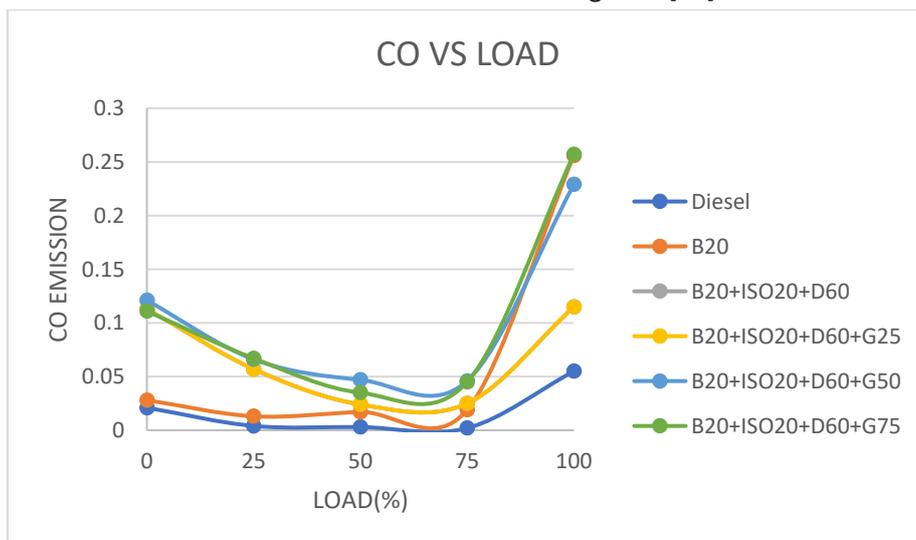
Fig 7. CO vs load
