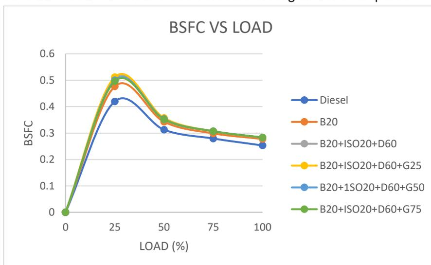
Fig 4. BSFC vs load
