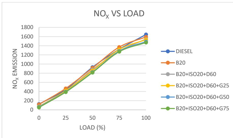
Fig 9. NO<sub>x</sub> vs load
