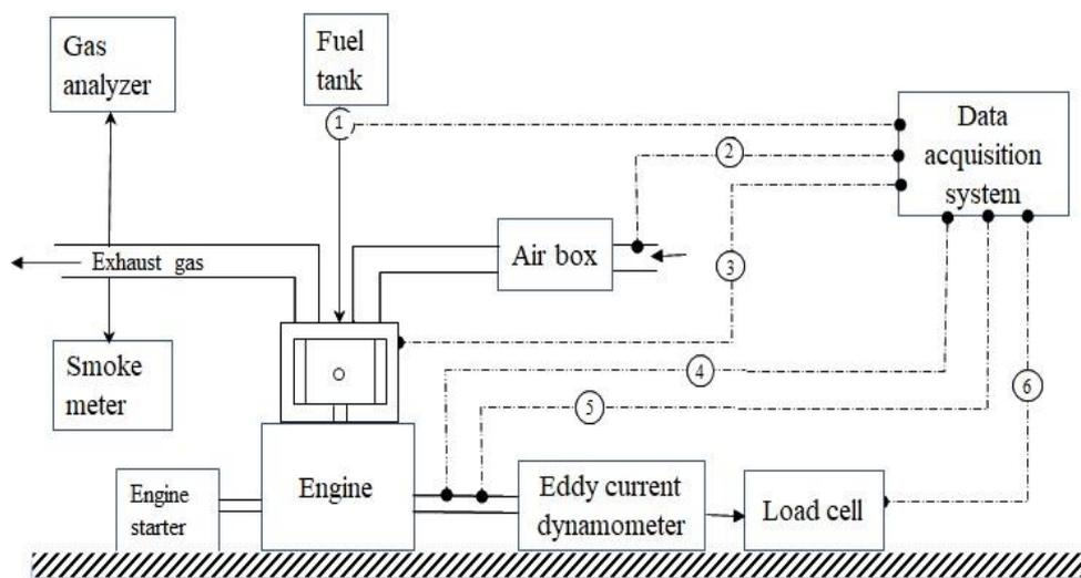
Fig1 Line diagram of CI Engine
