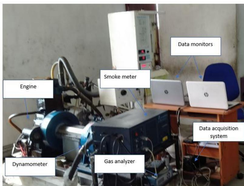
Fig 2. Photograph of CI Engine
