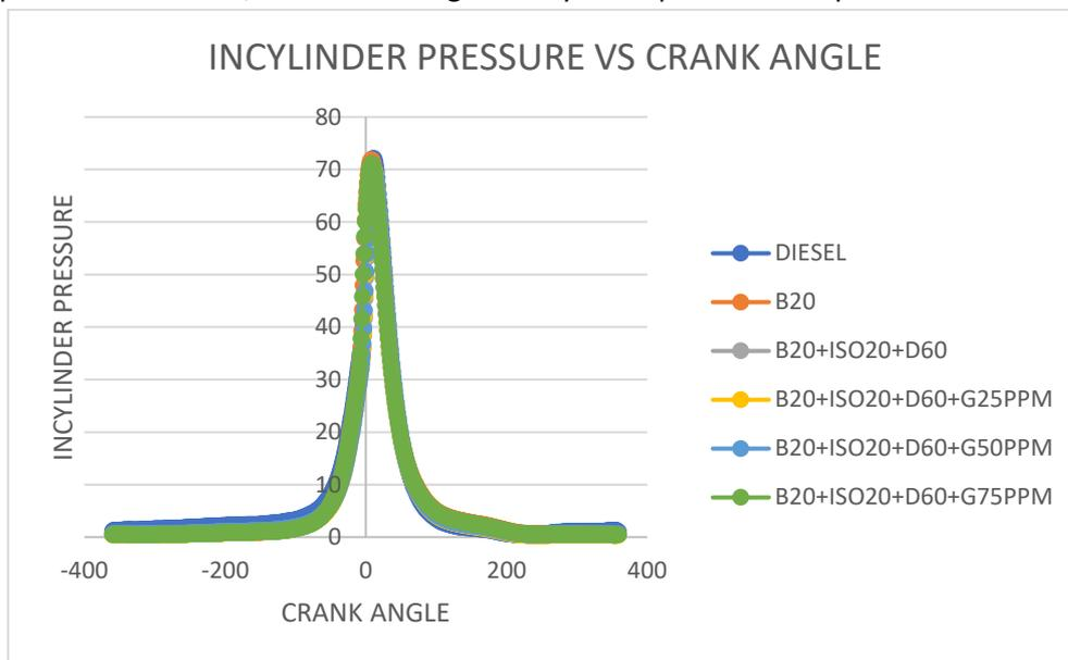
Fig 5. In-Cylinder pressure vs crank angle at full load
