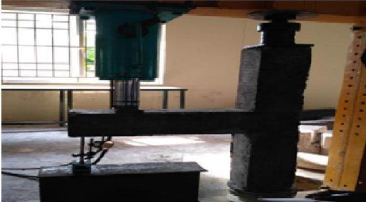
Figure 12. Cyclic load testing setup on L-section for downward load
