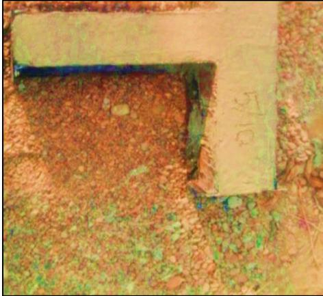
**Figure 9** Placing of GFRP mesh inside the mould and casting of L section specimen
