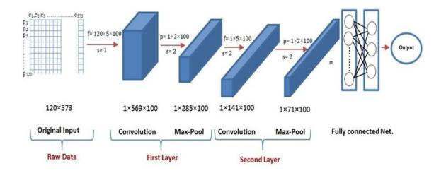
**Fig3.** The New Conceptualization Proposed Analysis of essential oil data begins with CNN using an original input matrix. The network's underlying structure consists of two convolution and pooling layers. Sigmoid activation is used in a fully connected feed forward neural network to select the correct output from these layers.
