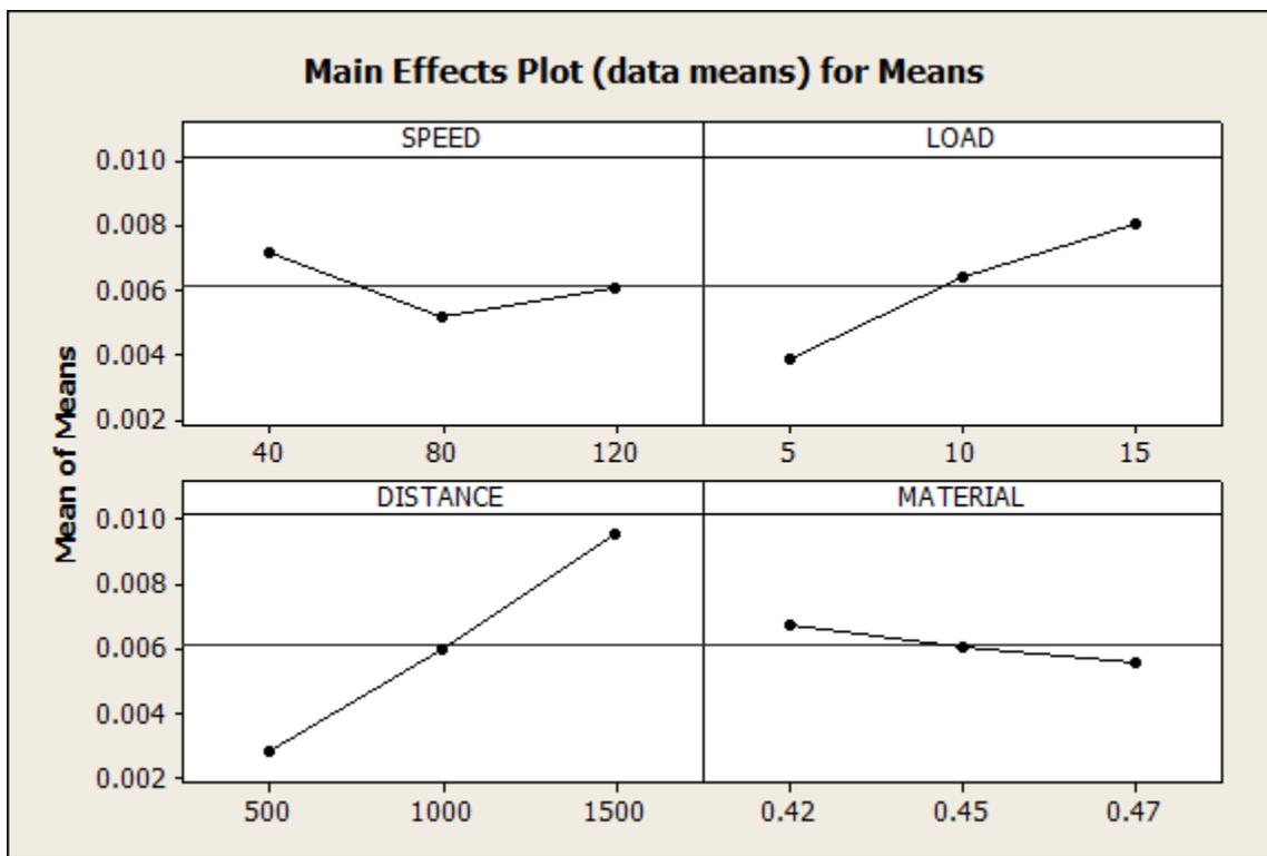
Fig. 2. Main effects plot for means- Weight loss
