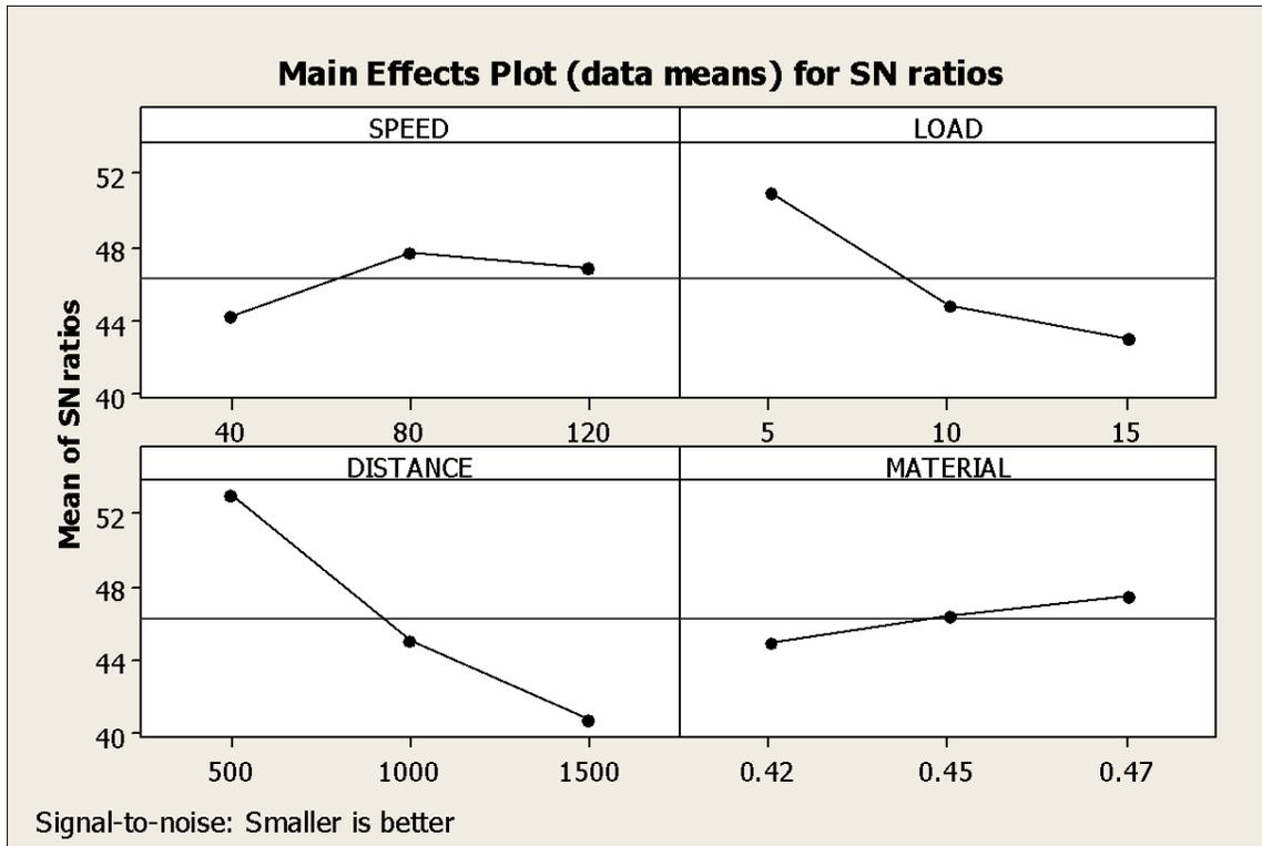
Fig. 3. Main effects plot for S/N Ratios-Weight loss
