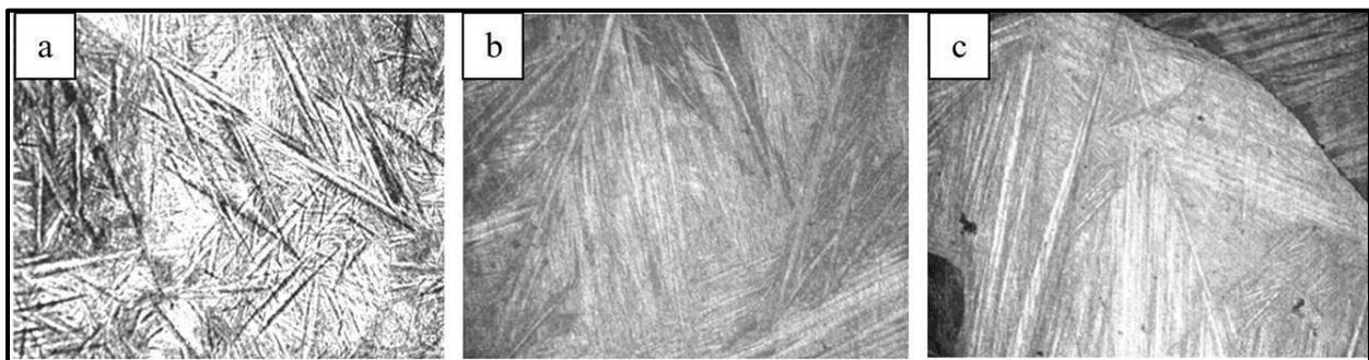
Fig. 1. Martensite observed for the composition (a) CAB1,(b) CAB2 and (c) CAB3
