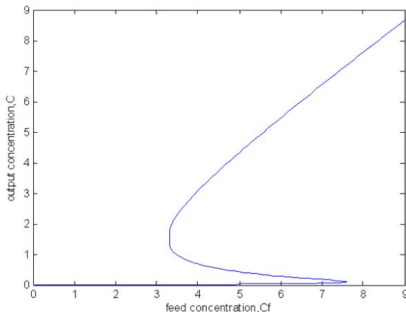
Fig. 2. Steady State Input-Output Map
