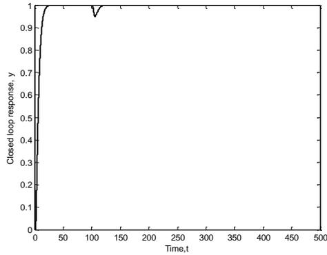
Fig. 9. Closed loop response for CSTR when input is in Region 3
