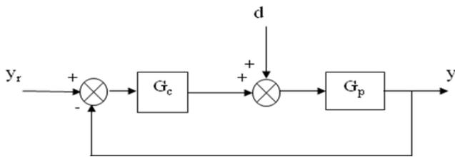
Fig. 1. Feedback control structure
