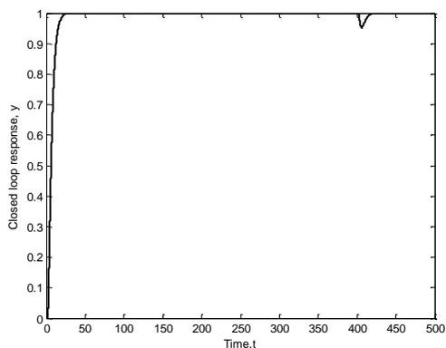
Fig. 10. Closed loop response for CSTR when input is in Region 4
