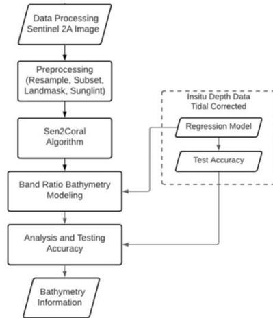
The estimated bathymetry value is determined from the processing of the three visible channels, namely the blue channel, the green channel and the red channel of the Sentinel 2A image. The resulted bathymetry values were then compared with each other to observe the differences that occur and then the accuracy of each bathymetric information extraction was calculated.
