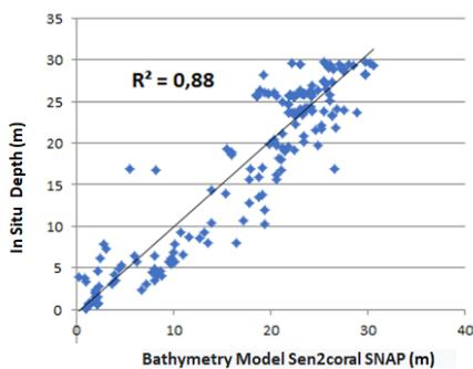
The validation of the satellite-based bathymetry model of the present study was conducted using 191 in-situ bathymetry data points collected during the field works. The accuracy of the model was assessed using several statistical indicators, including coefficient of determination ( $R^2$ ), root mean square (RMSE) and Kappa coefficient.
