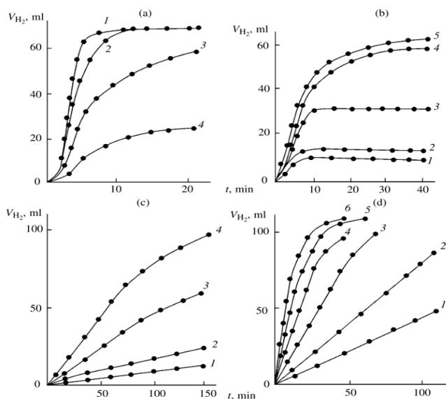
Looking at Fig10, the variation in the mass of aluminum and in the concentration of NaOH has exponential trends on the graph, for the variations in aluminum surface area has linear and quadratic trends, and for the temperature variations quadratic and exponential trends. Also, it was found that in the process of experiments that were at 20°C, with a very small aluminum mass of 0.02 g, and a concentration of NaOH 0.1 M, the volume of hydrogen was produced at 102.5 mL[17].
