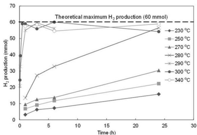
Previously, this research has been conducted by Aleksandrov et al. (2003), which uses metal hydrolysis methods for the production of hydrogen gas with various variations, namely in the mass of aluminum, the concentration of NaOH solution, the surface area of aluminum, and the temperature during the reaction. Graphs of volume production obtained from research, can be seen in Fig10, which shows almost the same patterns and tendencies in each variation.
