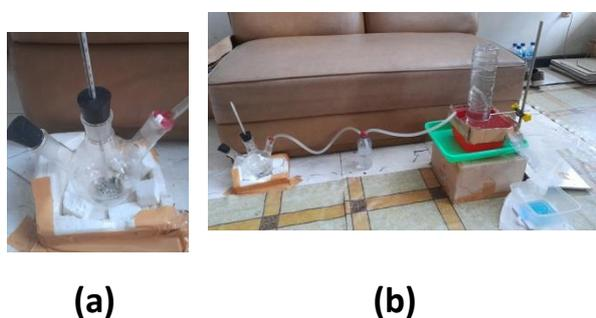
The hydrogen gas production volume was measured using the volume of water spilled into a container where water is spilled every 1 minute. The calculation was stopped when there was no more drop of water dripping into the container. From there, the values of the calculated production volume were plotted in a volume vs. time graph.
