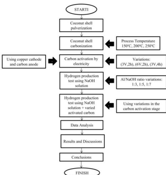
Fig1. Flow chart of the experimental steps for hydrogen production by hydrolysis process using catalysts and analysis.
