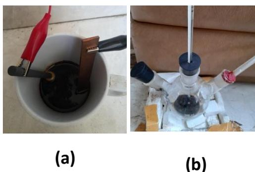
The hydrogen gas production process is carried out with the exact same set of equipment in Fig4(b), and the method of volume measurement was by using the volume of water spilled into a container where water is spilled every 1 minute. The calculation was stopped when there was no more drop of water dripping into the container. From there, the values of the calculated production volume were plotted in a volume vs. time graph.
