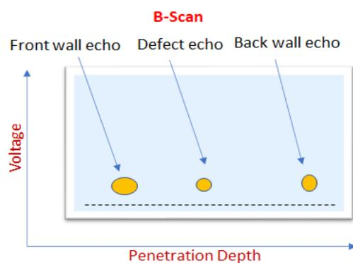
Figure 1.1 Method of B Scan UT
