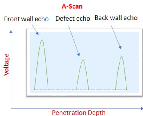
Figure 1.1 Method of A Scan UT echoes are displayed as dots on the CRO shown in the image[29].
