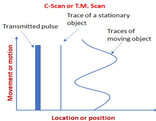
Figure 1.1 Method of C- Scan UT
