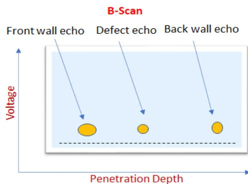
Figure 1.1 Method of B Scan UT
