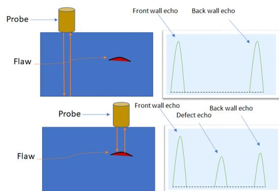
Figure 1 Method of ultrasonic testing
