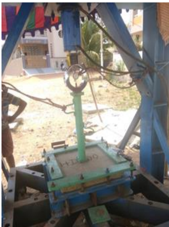
Figure 2: Test set up for testing of slab specimen
