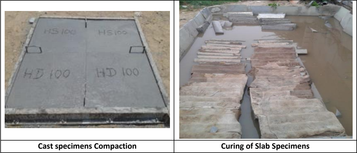
Figure 1: Casting and curing of slab specimens
