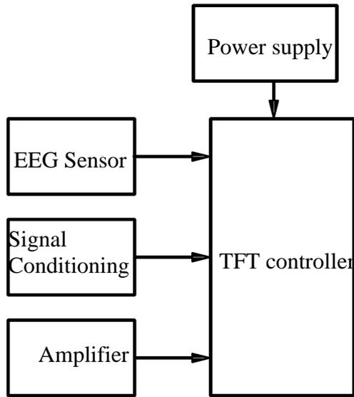
**Figure 4.2: SENSORS ARCHITECTURE**
