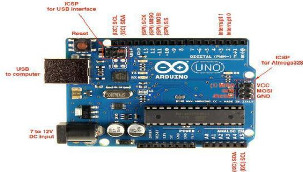
**Figure 5.3: ARDUINO UNO BOARD**
