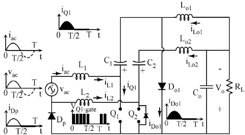
**STAGE 3:** During this interval, only the diode  $D_p$  conducts to provide a path for  $i_{L1}$ . Accordingly, the inductors in this interval behave as constant current sources. Hence, the voltage across the three inductors is zero. The capacitor  $C_1$  is being charged by the inductor current  $i_{L1}$ . This period ends when  $Q_1$  is turned ON.
