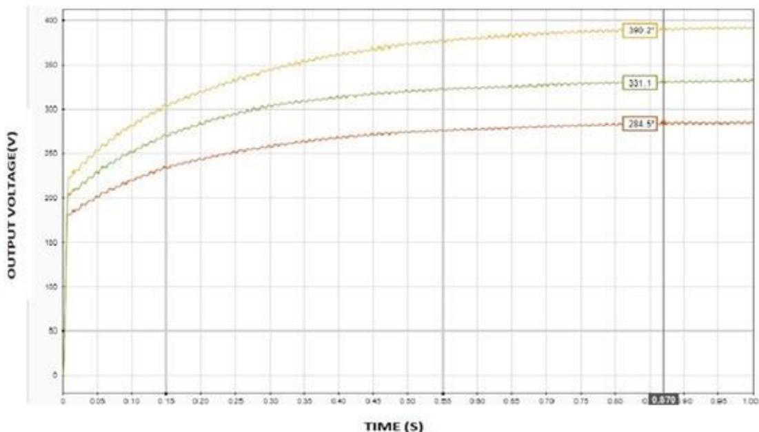
Simulation of EV charger in constant current control with disturbance.
