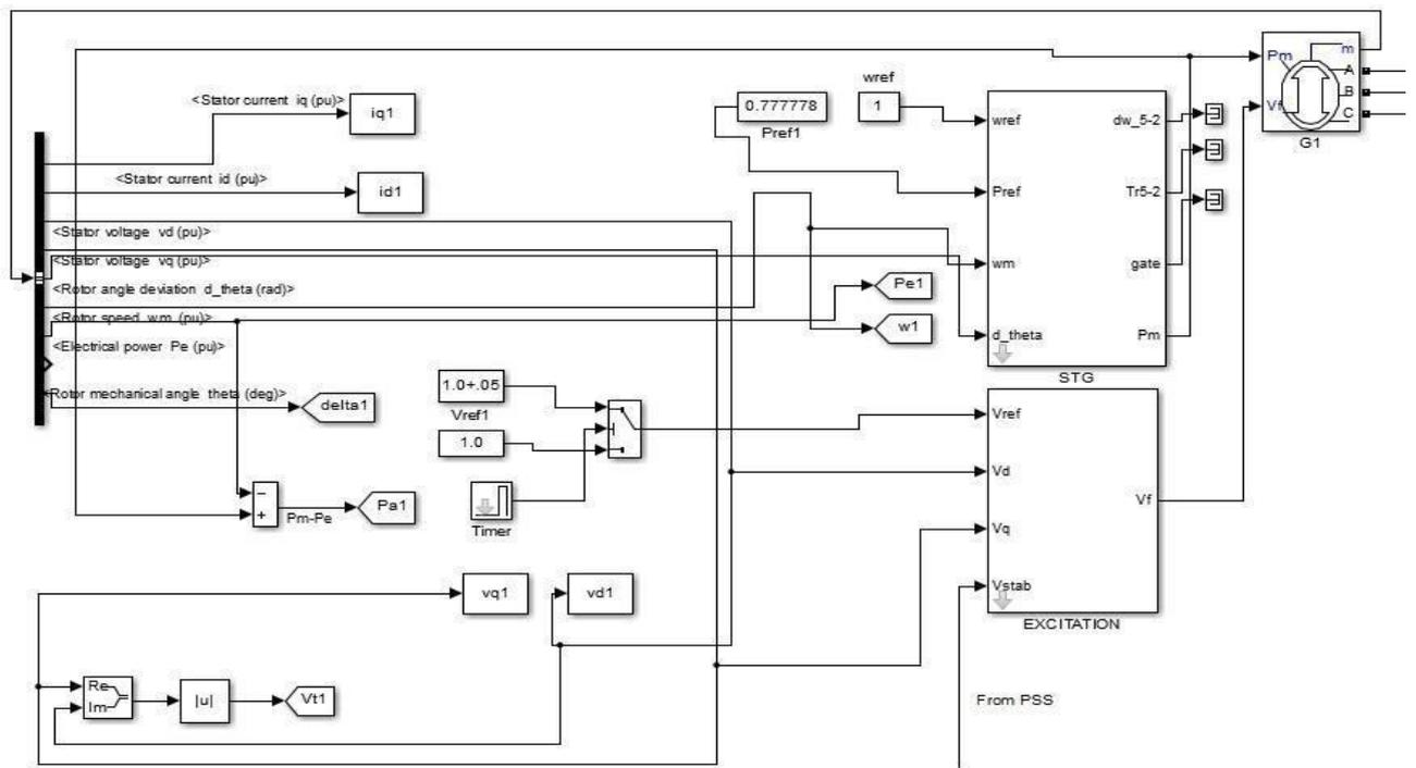
Fig. 1.7 Components used for each generator
