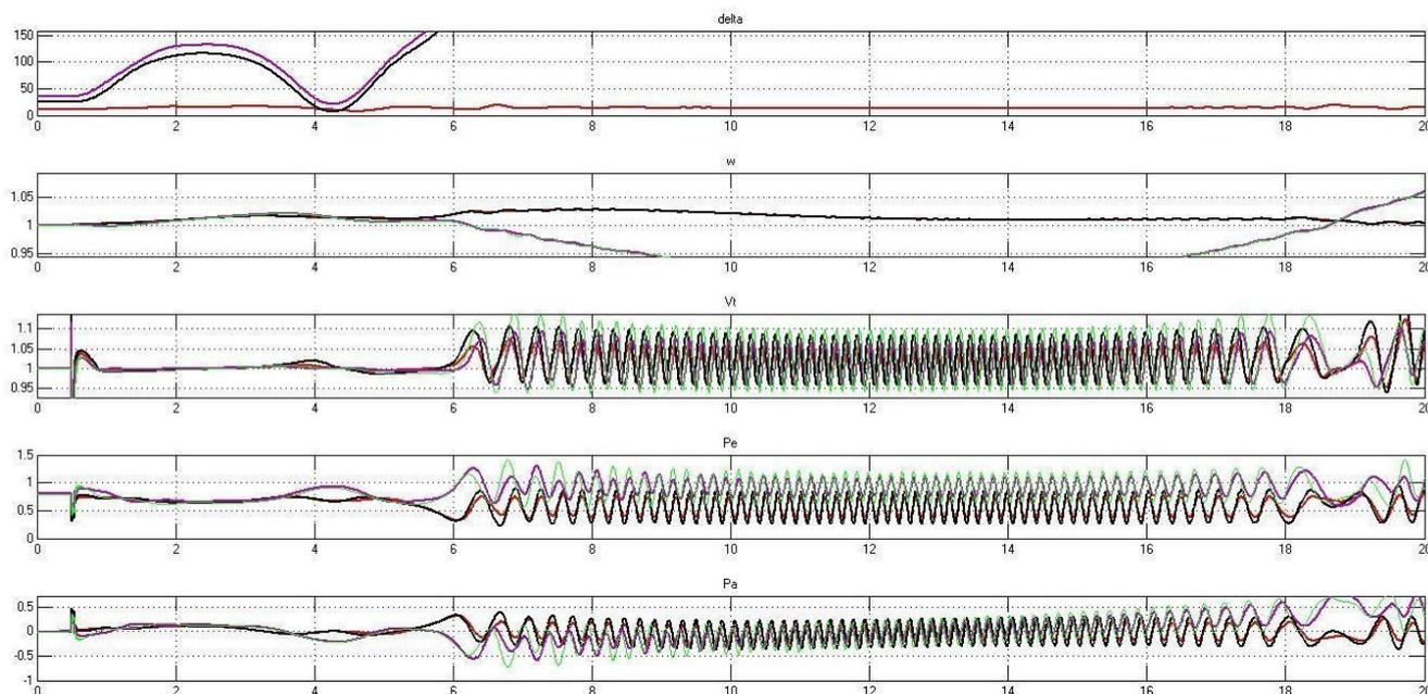
**Fig 1.9 Effect of 3phase fault on middle of one of the double circuit line without PSS**
