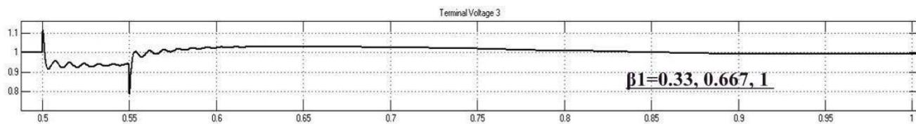
Fig.1.12 Terminal voltage for  $\beta_2=0.33$  and vary  $\beta_1$  from 0 to 1
