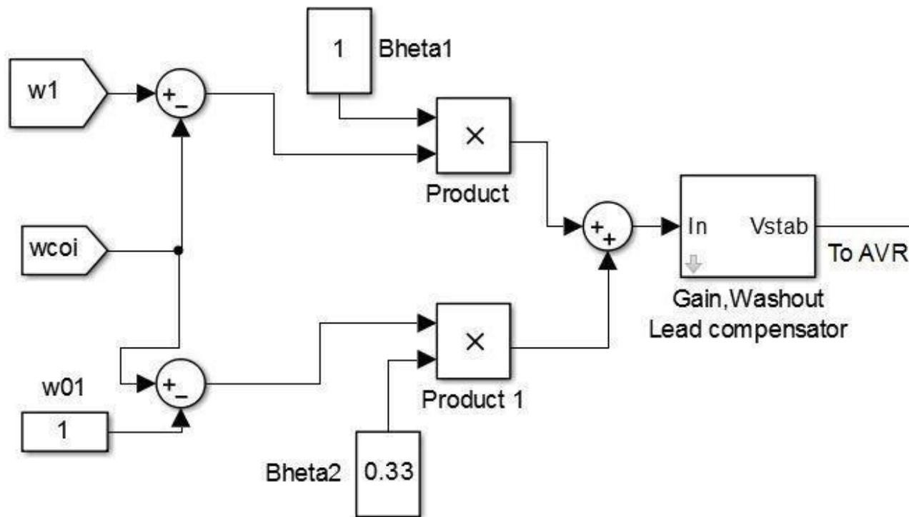
Fig 1.8 Generalized  $\Delta\omega$  PSS as simu link model
