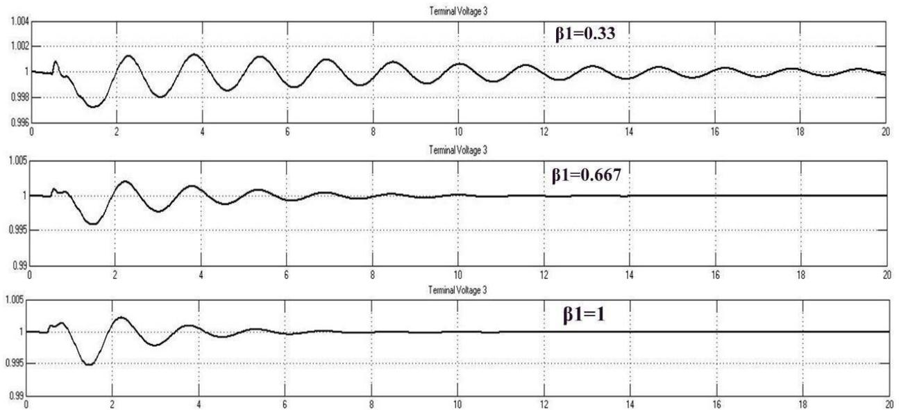
**Fig. 4.15 Terminal voltage of G3 for  $\beta_2=0.33$  and vary  $\beta_1$  from 0 to 1**
