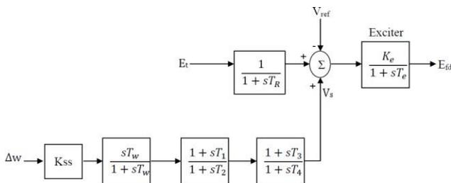
**Fig. 1.2 Conventional  $\Delta\omega$ -type stabilizer**
