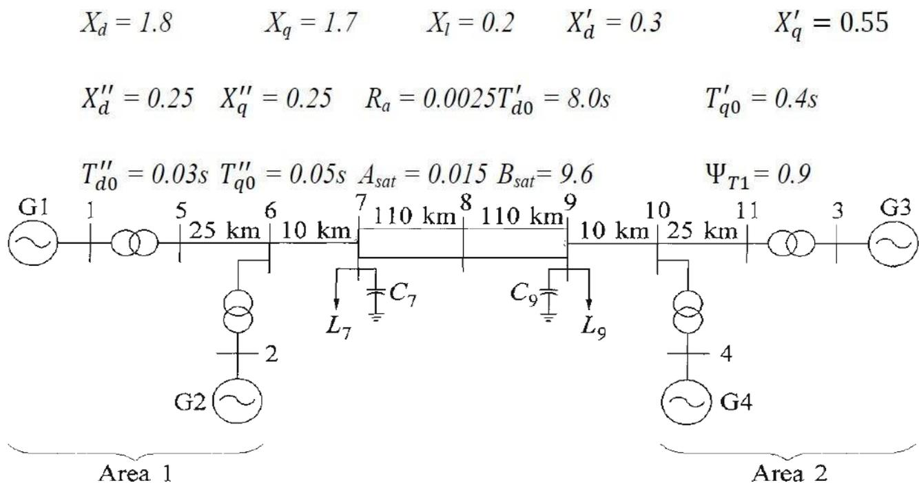
**Fig 1.5 Two-area system line diagram**
