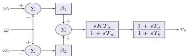
**Fig. 1.3 Generalized  $\Delta\omega$ -type PSS block diagram.**
