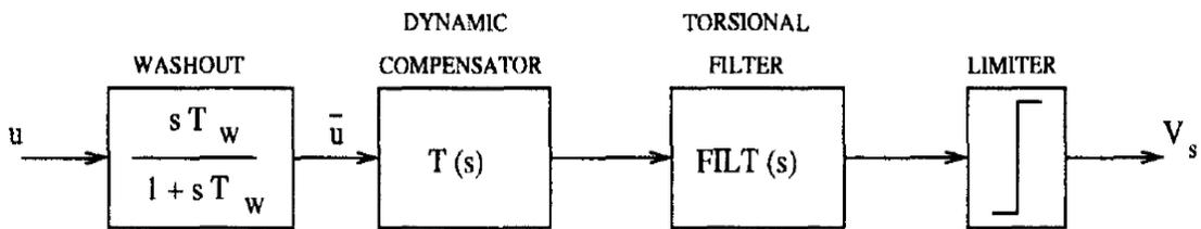
**Fig.1.1 Basic block diagram of PSS**
