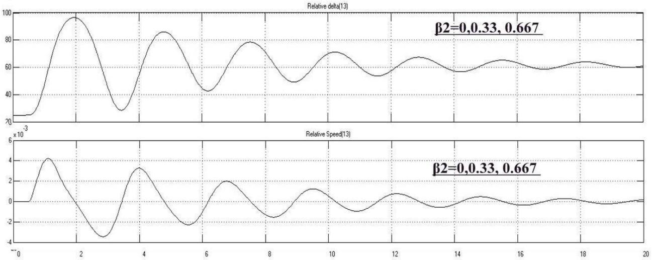
Fig. 4.8 Relative delta and relative speed for  $\beta_1=0.33$  and vary  $\beta_2$  from 0 to 1
