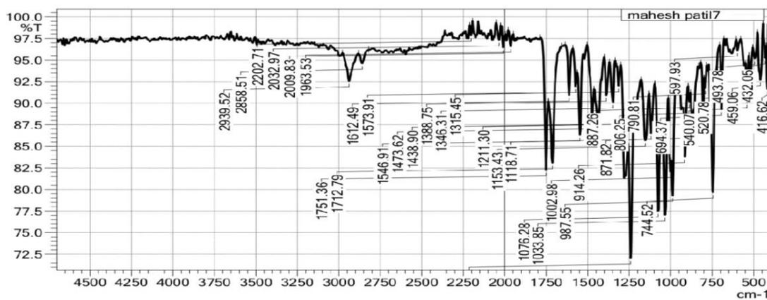
Figure 3: FTIR of physical mixture of candesartan cilexetil & polymers
