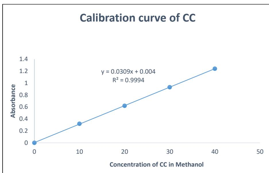
Figure1: Calibration curve of Candesartan Cilexetil
