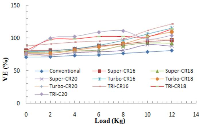
low, part and full load capacity with variation in compression ratio. For 12 kg of full load capacity, the VE increases from 81.17 % to 96.77 % for super CR16, 115.65 for turbo CR 16 and 121.88 % for tri-charged CR 16. Thus the higher value of VE at a compression ratio of 16 for super, turbo, and tri-charged engine (Fig. 10).
