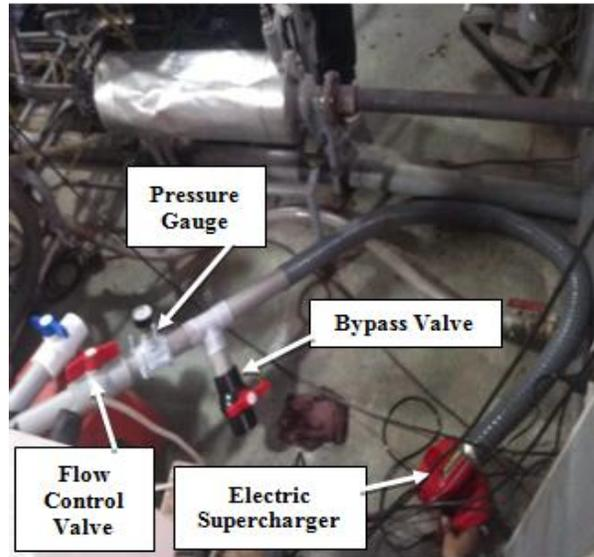
Figure 7. Tri-charged Engine Setup
