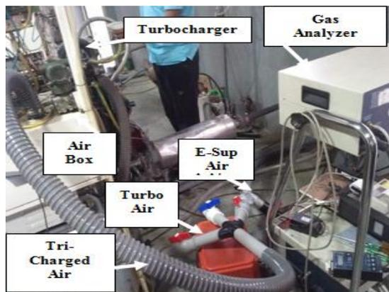
Figure 6. Electric Driven Supercharged Engine Setup
