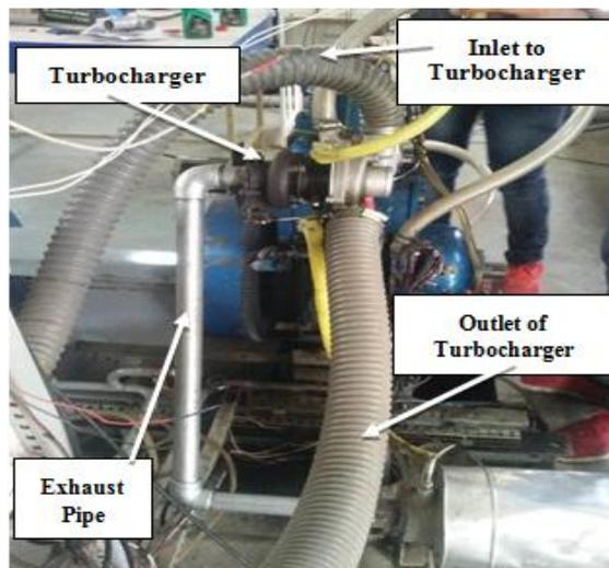
Figure 5. Turbocharged Engine Setup
