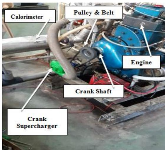
**Figure 4. Crank Driven Supercharged Engine Setup**
