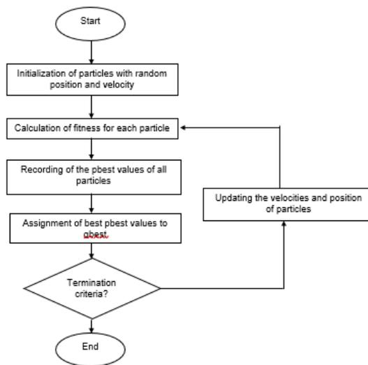
Fig. 6 Flowchart of PSO algorithm
