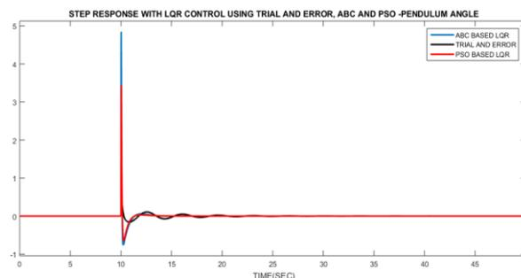
Fig. 11 Step response of LQR control for pendulum angle
