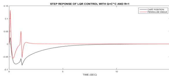
Fig. 9 Step response with LQR control
