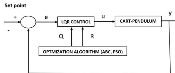
Fig. 4 Block diagram of LQR controller for cart pendulum system
