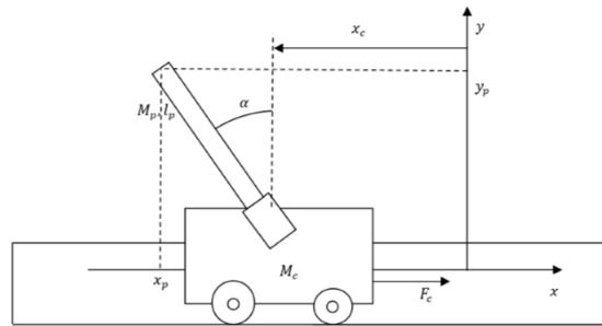
Fig. 2 Cartesian co-ordinates of Cart-Inverted Pendulum System
