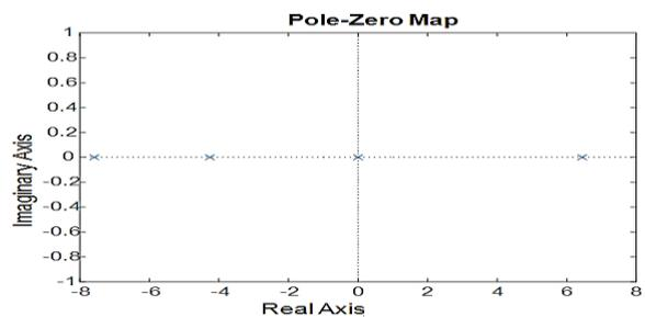
Fig. 3 Pole zero map of the cart-pendulum system model
