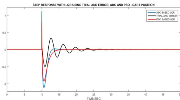
Fig. 10 Step response of LQR control for cart position
